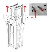
5. Remove the screws marked on the image then pull out the pulley system.
