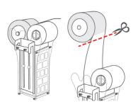
2. Press the red button to make the new fleece roll onto the motor, once it is attached to the motor, cut it off.
