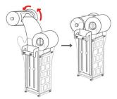
6. Fold the end of fleece into a triangle and place into the slot on the motor. Spin the motor to help it catch, then install the motor and press the red button to tighten the roll down.
