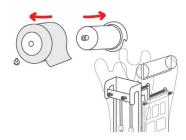
2. Pick up the motor and loosen the screw on the cover of the motor and separate the dirty
