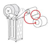
1. Pick up the old fleece roll, staple the end side with a new fleece roll, then place the new spool onto the filter.
