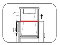
2. The main chamber will fill with bubbles. Carefully adjust the position of the collection cup by changing the position of the O-Ring. If you prefer the skimmate to be lighter lower the cup, and if you prefer it to be darker adjust the cup to be higher.
