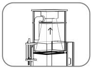
1. Pull out the venturi, and remove the collection cup.
