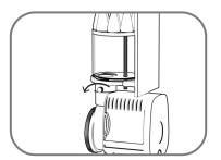
1. Loosen the screw under the diffuser and seperate the pump.
