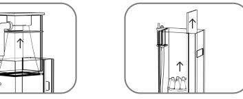
2. Pull out the inside plate and motor assembly and set aside.
