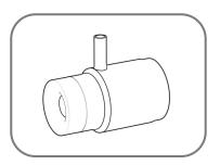
The venturi should be cleaned monthly and flushed weekly due to calcuim carbonate buikdup for best performance.
