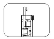
4. Reinstall the inside plate, venturi and coillection cup.
