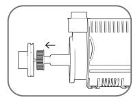
Remove the impeller and clean with warm water and aquarium-use toothbrush.
