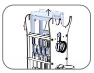
2. Lift both sides of the pulley system out of the main body assembly.
