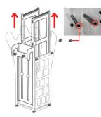
5. Remove the screws marked on the image then pull out the pulley system.
