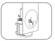
Loosen the screw on the pump collar to remove the pump.
