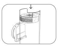
3. Place the sponges back into unit. (skip if using Biopellets).
