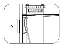
7. Use magnet to secure the reactor in its intended location.
