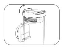
4. Replace lid and turn clockwise to tighten. (Do not over-tighten)
