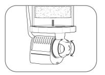
8. Set the flow control on the pump to the lowest setting, then plug in and adjust up to the desired flow rate.
